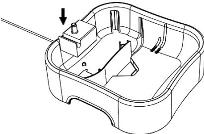
2.Put the wireless water pump into the corresponding place inside the water storage tank, and pay attention to keep the direction of the water pump consistent with the schematic diagram.
