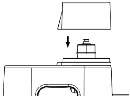
6.Place the water outlet platform T on the water outlet platform M.
