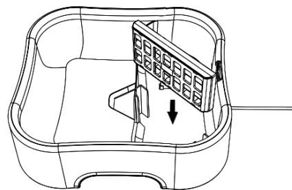
4.Place the water outlet platform B on the bottom shell. First clamp the buckle at 1 place, then clamp the buckle at 2 places. Then insert the ultrafiltration filter element into the water outlet platform B.
